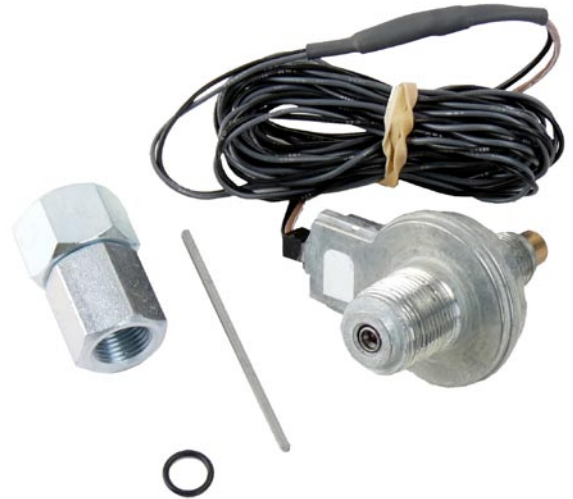
This aftermarket variable reluctance speed signal generator will send a pulsed speed signal to the GM PCM from the transfer case speedometer gear, while allowing for speedometer cable pass-through if you're retaining your factory mechanical speedometer.
