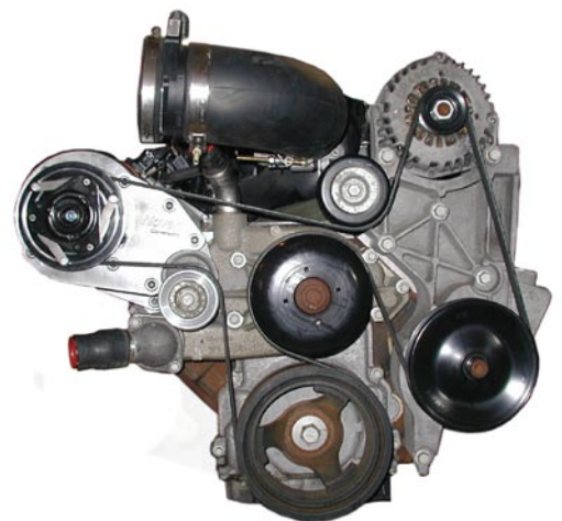
The Novak Gen. III+ A/C relocation kit, as assembled.
