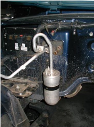
Remove the air conditioning dryer / receiver by detaching the bracket and removing the spring clip.
