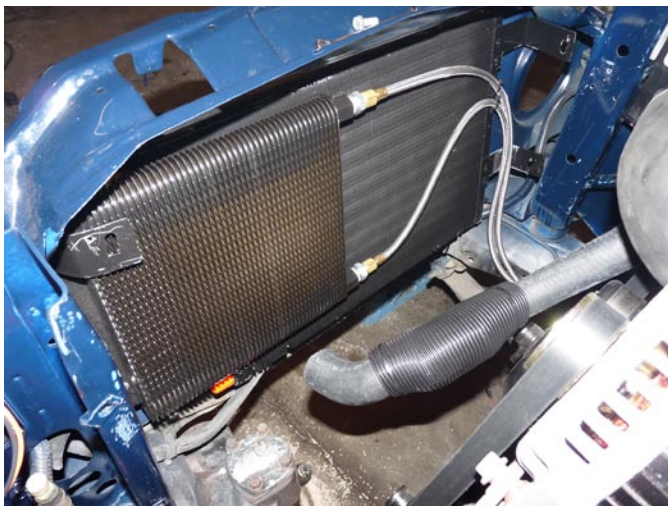
Both the A/C condenser and transmission cooler are placed in the generous space in front of the radiator and behind the grille.
